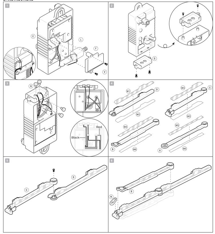
1. Insert the motor (L) into the main body (E). Place the motor wires into the slots then add the motor cover (F) and secure it with two screws (V).
