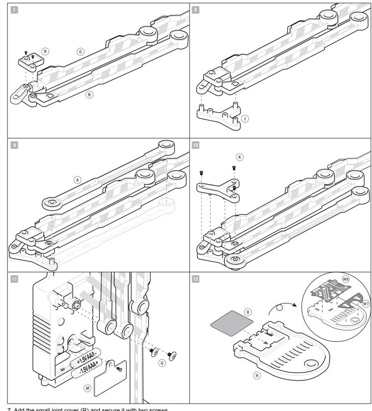
7. Add the small joint cover (R) and secure it with two screws. 8. Place the assembled arms onto the joint base (J).
