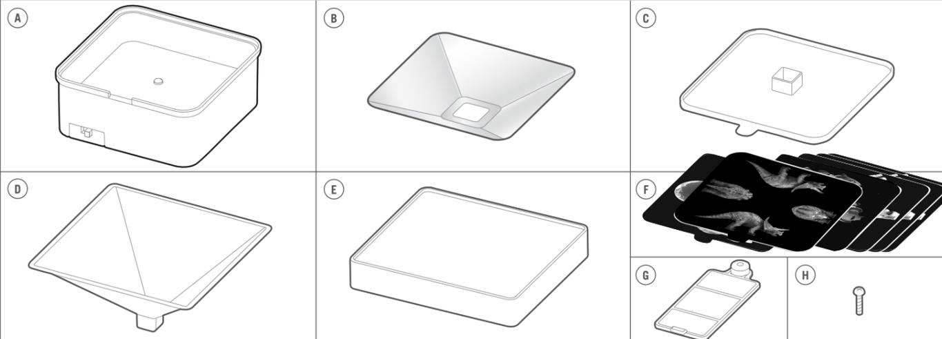
Part A: Base x 1, Part B: Reflector x 1, Part C: Transparent cover x 1, Part D: Four-sided screen x 1, Part E: Stand x 1, Part F: Paper template x 8, Part G: Battery cover x 1, Part H: Screw. Also required but not included: 2 x 1.5V AAA batteries and a small crosshead screwdriver.
