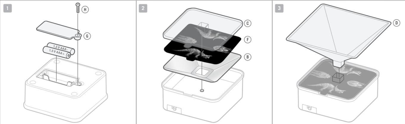
1. Turn the base upside down. Insert two AAA 1.5-volt batteries into the battery compartment, with the flat end of the battery against the coiled spring inside the compartment. Put on the battery compartment cover and secure it with a screw.
