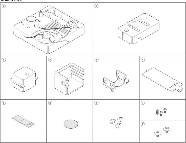
Part G: Adhesive tape, Part H: Metal disc x 1, Part I, Terminal caps x 3, Part J: Screws x 3, Part K: Washer screws x 2. Also required but not included in the kit: 2 x 1.5-volt AAA batteries, a small crosshead screwdriver.
